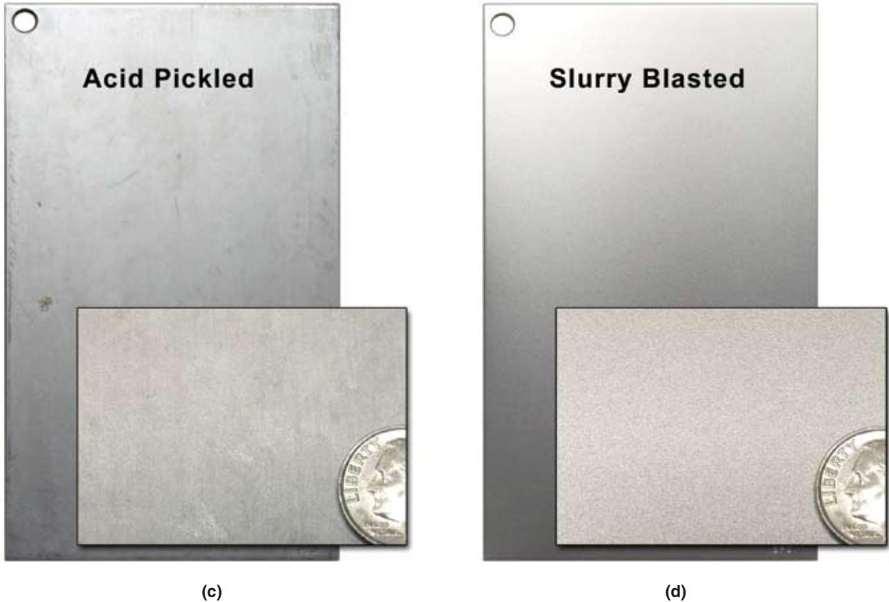
Views of surface treatments applied to hot rolled strip: (c) acid pickled and (d) slurry blasted.
