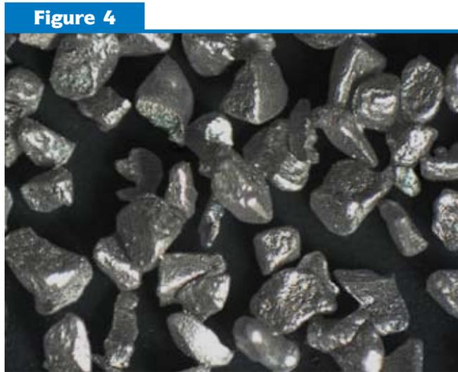
Carbon steel grit after conditioning by slurry blasting.
