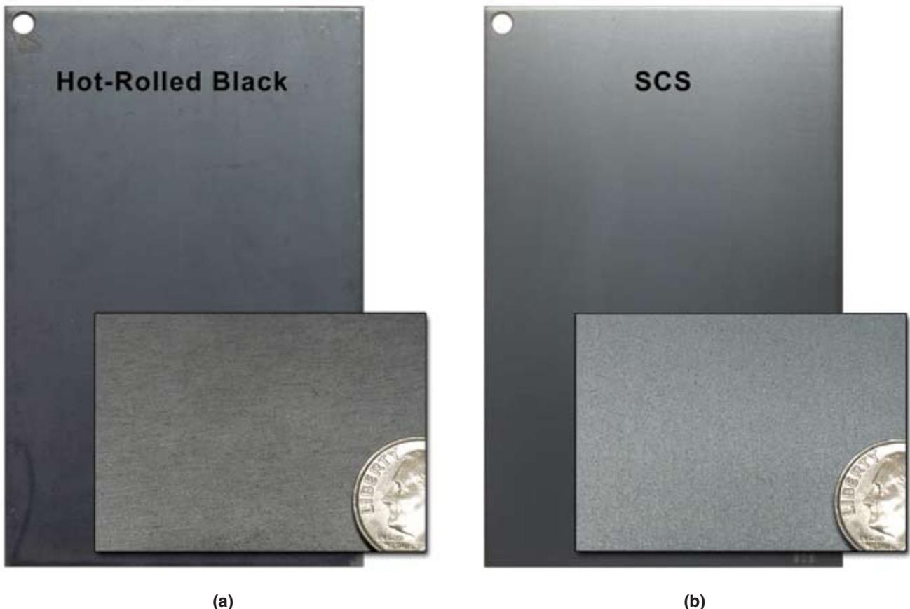
Views of surface treatments applied to hot rolled strip: (a) hot rolled black and (b) SCS.
