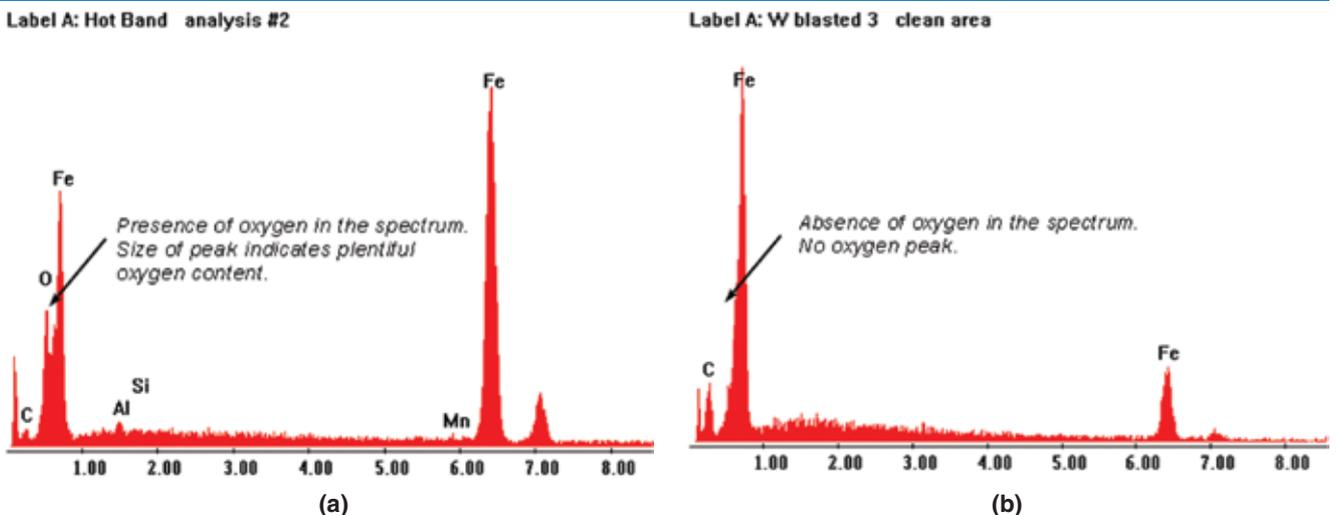
EDX spectra analyses: (a) pre-blast and (b) post-blast.
