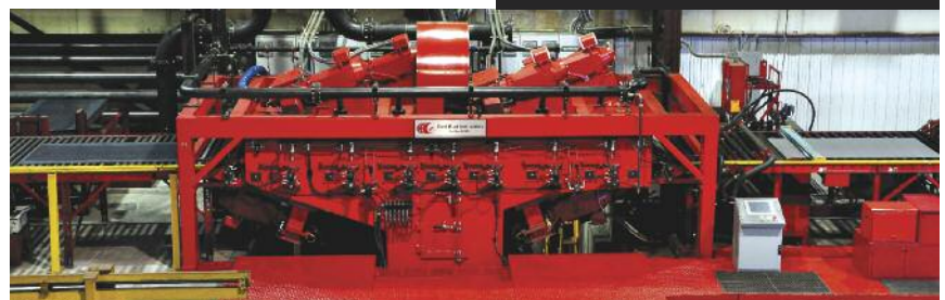
The special slurry solution in the chamber of TMW's eco-friendly EPS system reduces smut and doubles as a water-based rust inhibitor.
