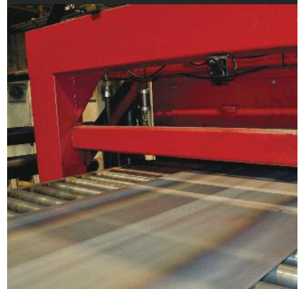
Kloeckner hot-roll black entering the EPS processing chamber for "pickling."
