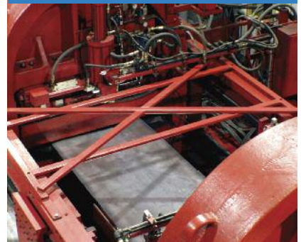
Kloeckner material is flattened through the stretcher leveling section of TMW's line, eliminating residual stress.
