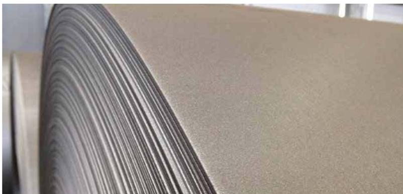
Hot rolled steel strip after EPS pickling
