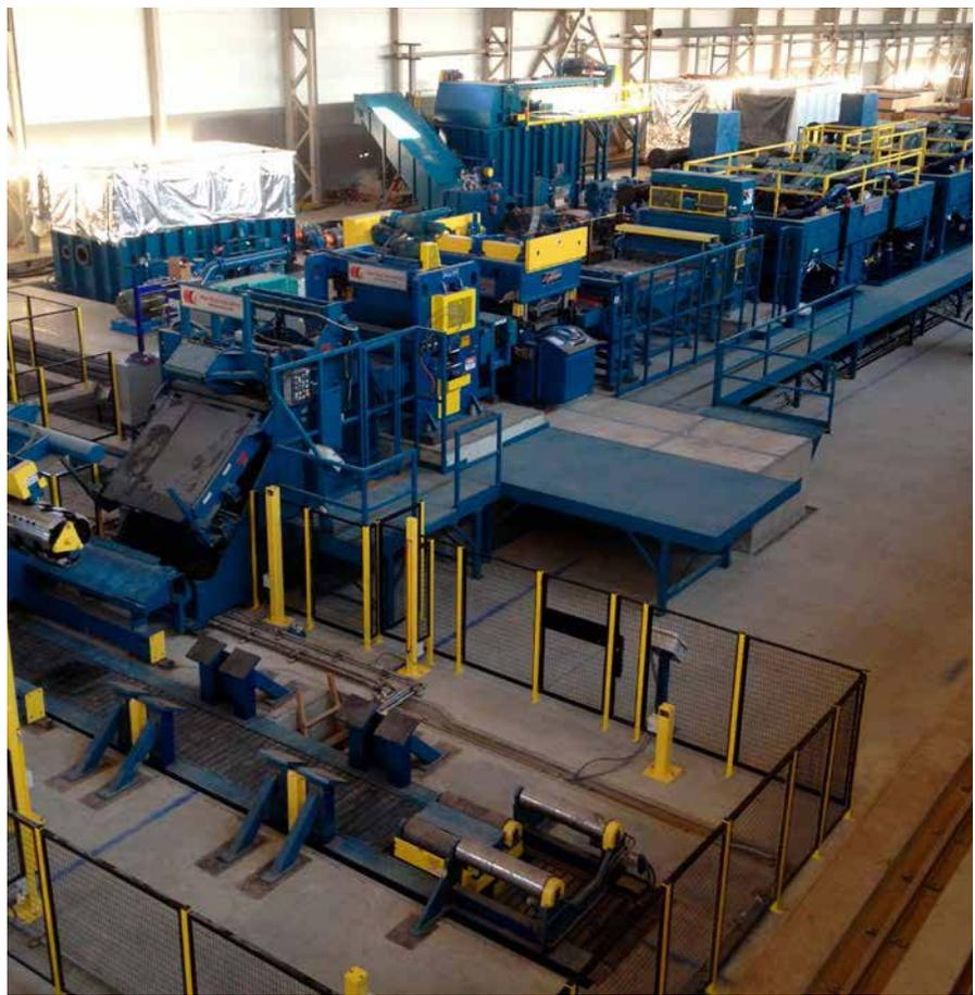
Metall Profil's EPS pickling line has two cells.
